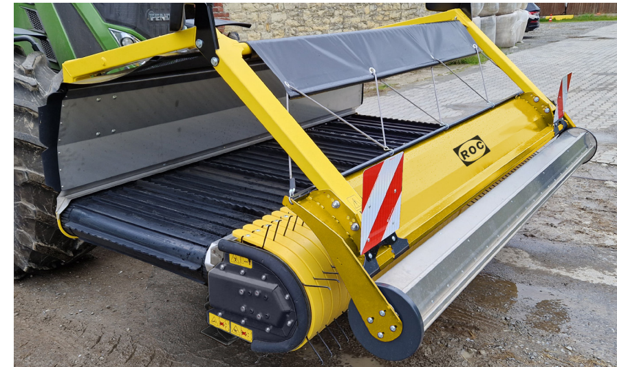
Working width 3.8m (12'6") and transport width 2.95m (9'8").
