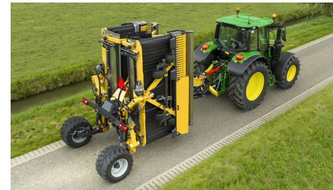
The ROC RS 730 can be folded into a width of only 2.5m for road transport.
