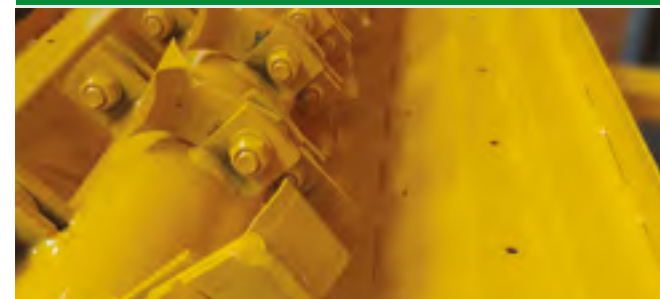
Self-cleaning roller position unloading of mulched product behind the roller for faster working speed
