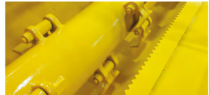
Position of the self-cleaning rear roller for discharging the mulched product behind the roller for higher output
